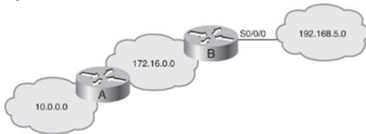
Figure 4-27. Network 10.0.0.0 Needs to Be Hidden from Network 192.168.5.0.
